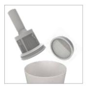
Tap the filter and separator against a bin to remove dirt and debris. Wipe over the separator metal shroud with a dry cloth.
