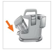
To re-fit, tilt the dirty water tank and line the front of the tank up onto spot washer. Push back until it clicks into place.
