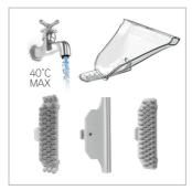
Rinse the attachments and the nozzle under warm water (max 40°C) to remove dirt/debris.
