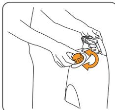
Tighten cap before returning tank to unit.
