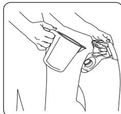
Fill clean water tank with solution mix.
