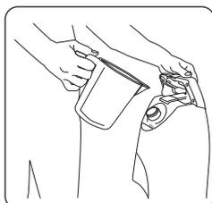
Fill clean water tank with solution mix.
