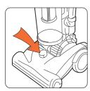
The front of the vacuum cleaner has a brushbar height adjuster that raises and lowers the brushbar to suit the type of carpet. With the cleaner NOT connected to the electrical outlet, and when the vacuum is in the upright position set the adjustment to the lowest setting for maximum cleaning. If the cleaner is difficult to move, push the knob to the next highest setting until the vacuum is comfortable to push. The brushbar must reach the carpet for effective cleaning.
