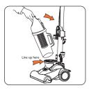
Insert the bottom of the dirt container to align with the tab on the upper cover of the motor. To secure the dirt container, push the top in place, there will be an audible click when it is secure.
