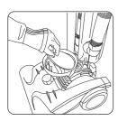
Underneath the dirt container is a pre-motor filter. If found to be defective, please replace.
