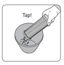
Firmly tap clean the HEPA filter until no more dust is observed falling out. The HEPA filter may be washed by running it under the tap. We recommend washing it once a month or when suction appears reduced. Always allow to air dry for 24 hours before replacing into the vacuum.
