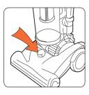
The front of the vacuum cleaner has a brushbar height adjuster that raises and lowers the brushbar to suit the type of carpet. With the cleaner NOT connected to the electrical outlet, and when the vacuum is in the upright position set the adjustment to the lowest setting for maximum cleaning. If the cleaner is difficult to move, push the knob to the next highest setting until the vacuum is comfortable to push. The brushbar must reach the carpet for effective cleaning.
