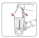
Remove the dirt container lid by grasping the dirt container and turning anti-clockwise.
