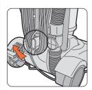
This vacuum cleaner is equipped with a convenient cord storage feature. The power cord winds around the two cord holders at the side of the unit. The bottom cord holder has a quick release feature. Turn the cord hook to the left or the right to remove the power cord.
