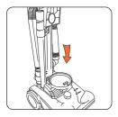
Firmly push the back panel onto the base assembly.
