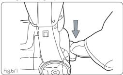
While depressing the solution spray trigger, pull carpet washer in a backward motion. Release the trigger and push the unit forward in the same path to agitate and remove dirty water and solution from carpet. (For more heavily soiled areas, repeat if necessary).
