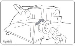
When finished cleaning remove the dirty water tank and rinse with warm water and allow it to dry before storage. Also remove filter (as shown) rinse with warm water (max 40°C) and allow it to dry thoroughly before storing.
