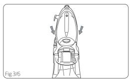
Line up mid-section with base unit and slot into place (Fig 3/6).
