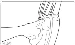
Unscrew the measuring cap from the reverse side of the clean water tank. Fill measuring cap with solution (Use only 1 capful of solution per full tank). Pour into clean water tank (Fig 5/2).
