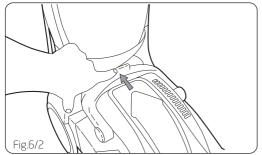
Twist dirty water tank outlet cap to the left and remove, empty, rinse and replace (Fig.6/3)
