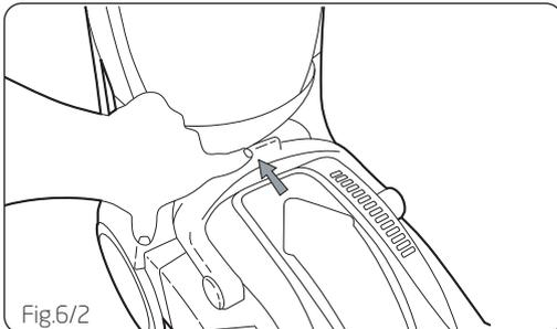
Twist dirty water tank outlet cap to the left and remove, empty, rinse and replace (Fig.6/3)
