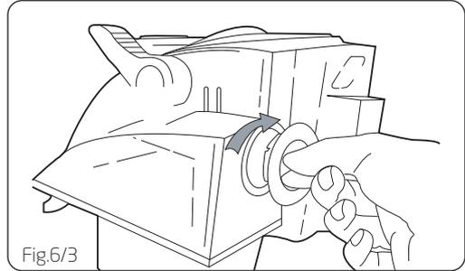
When finished cleaning remove the dirty water tank and rinse with warm water and allow it to dry before storage. Also remove filter (as shown) rinse with warm water (max 40°C) and allow it to dry thoroughly before storing.
