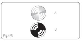
**NOTE:** If the indicator does not spin and the pattern is visible (B) when the carpet cleaner is turned ON, the brushes are not rotating.
