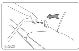
Turn carpet cleaner on. If necessary, refer to "Before using tool" section to remove air from system.
