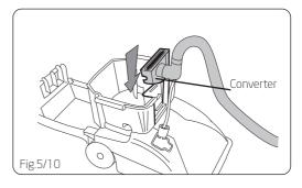
**NOTE:** Before connecting tube to cleaner, make sure black tabs are extended by pulling tan collar toward tube.
