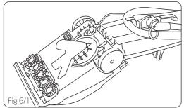
Grasp inner portion of brush and pull brush assembly out slightly to reveal latches (Fig 6/2).
