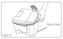
The lid replaces in a hinge-like manner. Position the front of lid under tabs on front of tank. Rotate lid down onto tank.
