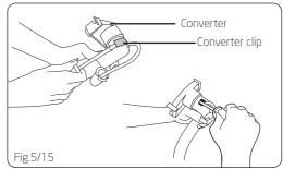
Snap clip back into position making sure solution hose is not pinched and moves freely (Fig 5/16).
