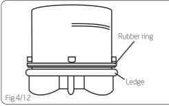
Replace cap. Rotate cap clockwise until it locks in place.
