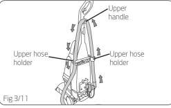
Wrap hose around lower tool holder and continue until nozzle connector is near upper hose holder.
