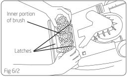
Press all four latches and pull brush block out. The brushes can be cleaned under running water (Fig 6/3).
