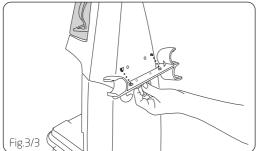
Place nuts in recessed areas on back of hose holder. Hold each nut in place while tightening each bolt securely (from the front of the handle) with a Phillips screwdriver. Only two nuts are needed on this model. The extra nut is not required but has been provided for your convenience (Fig3/4).
