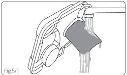
**NOTE:** If the filter must be removed for cleaning, it is easier to replace if the filter is wet.
