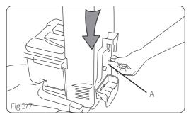
Replace clean solution tank (upper tank) by positioning bottom first.
