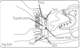
Press brush assembly firmly to snap into place (Fig 6/5).
