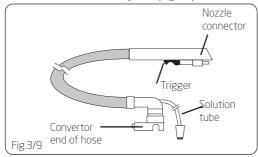
Start with converter end of hose. Fit converter over tab near tool holder.
