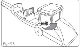
Unlatch back part of tank lid and remove lid. Empty tank. Pour dirty water out from the rear of the tank (Fig4/16).
