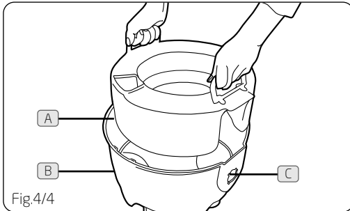
Fig.4/4 5. Replace Motor Container (A) ensuring that the Solution Pump Hose (B) is aligned with the hole in the Clean Water Tank (C) so that it goes inside when the Motor Container is clipped back into position (Fig.4/5).
