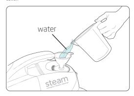
If the water tank needs to be refilled during use, first switch the cleaner off and remove the plug from the socket. Before opening the tank cover to refill the tank, release the steam switch on the steam gun or allow the cleaner to cool down completely.
