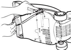
Grasp the brush bar with one hand, using the other hand to keep tension on the the belt while removing.
