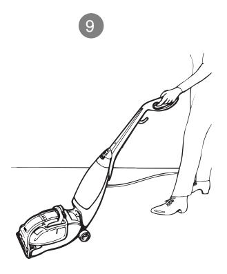
Plug the cord into a mains electricity socket. Turn the power and brush bar switches on. The switches are located on the front of the cleaner, above the solution reservoir. The power switch controls the vacuum motor and pump, the brush switch only turns the rotating brush
