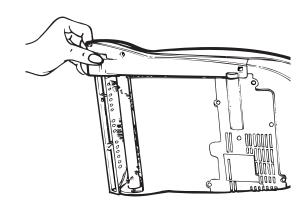
When replacing the belt, first slide it onto the motor shaft. Then slip the brush bar through the belt. Place the belt in the area of the brush without bristles.
