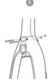
Place a nut into the recess in the back of the upper handle. While holding the nut in place insert one of the large screws through the front of the upper handle and tighten.
