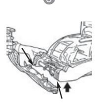
Return dirty water tank to the base of the cleaner by tipping the nozzle down into the basin and dropping it into place.
