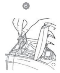
Dirty water tank can be rinsed out with hot tap water to remove any remaining debris. Wipe and let dry thoroughly before storing to prevent mildew from forming.
