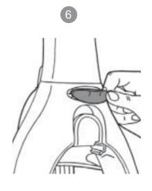
Remove the backing tape from the screw cover and press into place.
