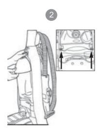
Line up the grooves of the clean water tank with the support posts inside the handle. Tilt the top of clean water tank inward and push until it locks into place.
