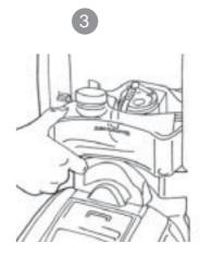
Remove the clean water tank by pressing the clean water tank release and pulling the tank by the handle. Put to one side to fill later.
