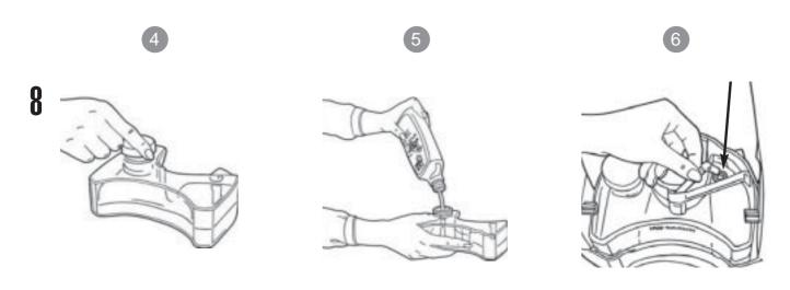
Remove solution tank cap.
