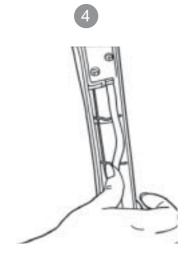
Feed the cord through the slots on the back of the handle and push into place.
