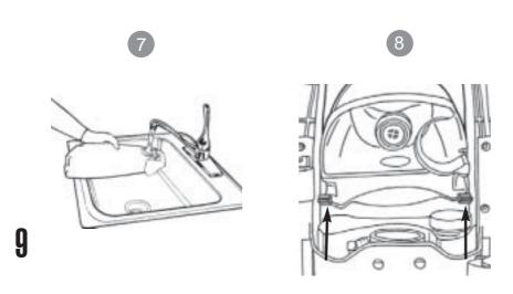
Remove the clean water tank cap and put in a safe place. Slowly fill the clean water tank with hot tap water and replace the cap.
