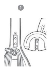
To install the tool caddy, line up the tabs of the tool caddy storage with round tabs on the back of the handle (above quick cord clip).
