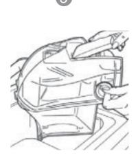
Depress the dirty water tank latch and simultaneously pull the dirty water tank nozzle tab up and away from the cleaner. Remove the dirty water tank by lifting the dirty water tank handle and pulling the tank out of the base.
