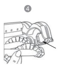
Tilt cleaner off the carpet. Grasp the brush bar and pull the right side of its chamber.
