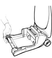
To empty the water tank grasp the handle with one hand and nozzle with the other and empty into the sink.
