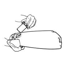
Unscrew the filler/ measure cap from the rear of the solution reservoir.
