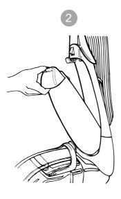
Tilt the solution reservoir away from the cleaner and remove.
