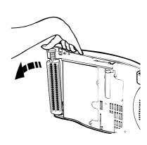
Remove the water tank switch off and unplug carpet washer.
