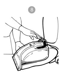
Grasp the handle and hook the front of the dirty water cleaner into the base, making sure that the front of the dirty water tank is resting on the base.
