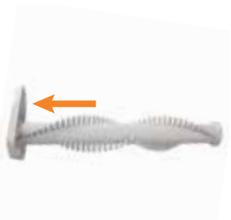
To re-fit the brushbar, firstly push the brushbar onto the brushbar cover, then slide the brushbar and cover back into the brushbar housing. Make sure the end of the brushbar sits securely in place. Refit and tighten the screws to secure.
