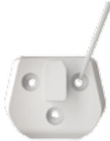
Align the bracket back to the wall and make an additional 3 small marks for each screw.
