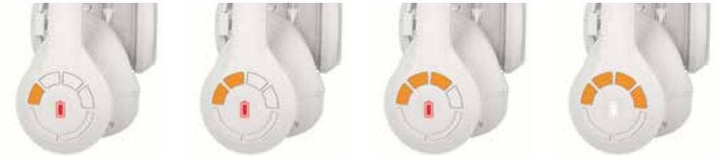
The battery level gauge lights will illuminate in turn as the battery charges, until all four lights are illuminated. Once fully charged, the gauge lights will go out and the central light will illuminate white. If charging for the first time the initial charge time is 4 hours.
