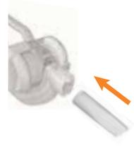
Push the chosen accessory into the handheld until it is securely locked into place.
