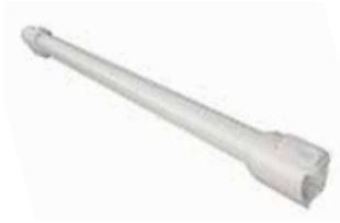
To test for a blockage in the reach wand, drop a small ball of paper into the wand. The paper will drop through if the wand is clear. Use a broom handle or similar blunt object to remove any blockage.
